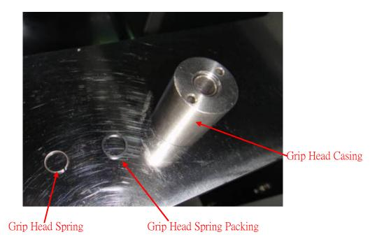
5. Install the casing on the bracket and make sure the spring with packing isn't apart from the casing during installation.
